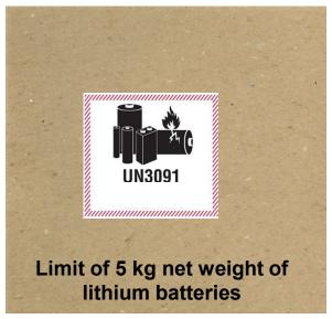
Section II Lithium Metal – 1 g/cell, 2 g/battery
